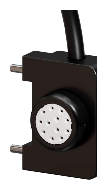
The SEK125 is a medium-sized module with IP40 protection. It can be used in various categories of manual robots, including SHW063, SHW080, SHW100 and SHW125, and has 12 electrical points.
