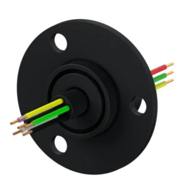
Slip ring specially suited to transmit critical signals, such as hi frequency and data rate, low current and voltages (strain gauges, thermocouples, measuring equipment, etc.) and offering a optionnal fieldbus or Ethernet channel (EtherCAT, Profinet, Profibus, etc.).
