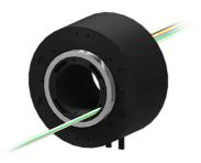
Slip ring for transmission of electrical power and/or electrical signals with through hole for shaft or rotary union. E1M/E1G option comes with an Ethernet channel (100BASE-TX or 1000BASE-T) over a Cat5e cable and 0P1/0P2 option offers an integrated pneumatic rotary joints and 6 to 24 power circuits.
