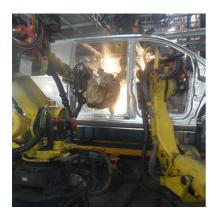
Flexible welding lines that we find in the automotive industry shall take up minimum floor space and then requires a single robot to often handle several welding guns.
