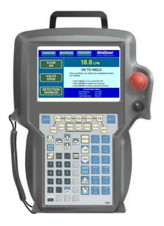
The WeldSaver graphical user interface provides information on device status in real time, with clear visual indicators and descriptions. The interface can be accessed over a network using most JavaScript<sup>TM</sup>-enabled web browsers by entering the working IP address of the device.
