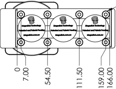
NOTE: For mounting of custom pole shoes, housing threading is 8X M8 X 1.25  $\nabla 10.00$  mm
