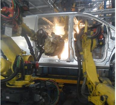
The welding gu in itself is concentration of technology, it embeds servo control of position and strain, the welding power and all the electronics and sensors needed to enable automation of the equipment. Wathan find
