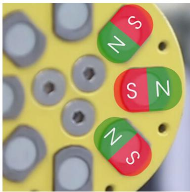
Robotic destacking of metal sheet with magnetic grippers may sometimes cause some issues. Indeed, the magnetic field may reach several sheets at a time and residual oil or other lubricants between successive sheets make them stick together.
