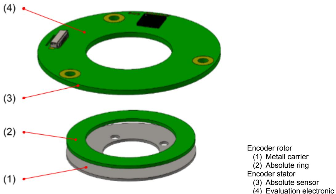
The absolute inductive sensor (3) scans the variable electrical impedance of the absolute ring (2) and generates an electrical signal. The inductive sensor (3) is connected to the evaluation electronic (4) which converts the electrical signal in digital position. Absolute
